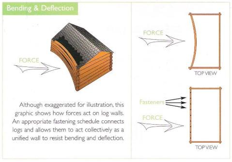
throughout the wall rather than just along one log. Acting similar to a built-up beam, the log wall transfers the lateral loads to the wall's bearing points (the corners, for example). Using a simple beam calculation, a designer can determine if the log wall can span from corner to corner or if it will need intermediate support (using interior walls or stiffening posts).
